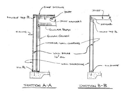
All spacings are set to 16" o.c., all support members are 2" nominal and all sheathing and decking is to be installed with strength axis perpendicular to supports (Three-Span Condition). Therefore:
